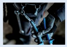
Correct attachment of the tool to the lanyard. **Return the tool to the belt following the steps in reverse order.**
