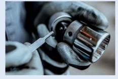
When mounting sockets or extensions make sure that the hole in the socket and the pin on the square drive are aligned. Using the socket remover (Article 1111) depress the pin while attaching the socket. Make sure that the pin clicks into the hole.
