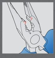
The pliers can be used for crimping insulated spade terminals.
